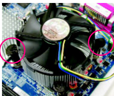
Fig. 3 Place the CPU cooler atop the CPU and make sure the push pins aim to the pin hole on the motherboard. Pressing down the push pins diagonally.
